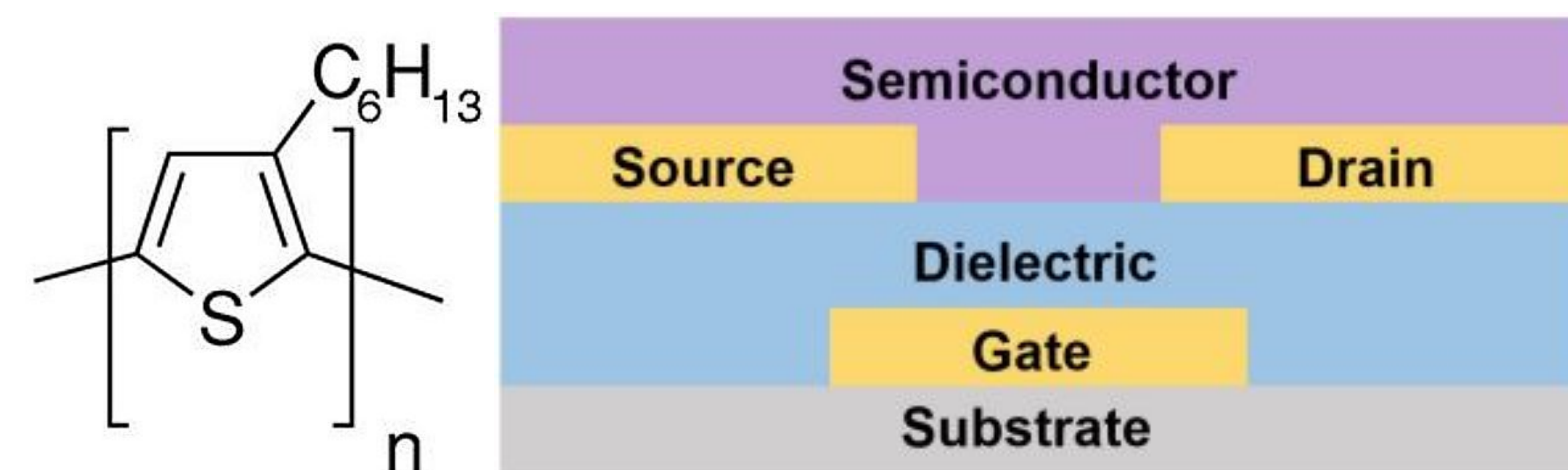
Fig. 1: Chemical structure of P3HT (left) and a schematic illustration of OFET (right)
