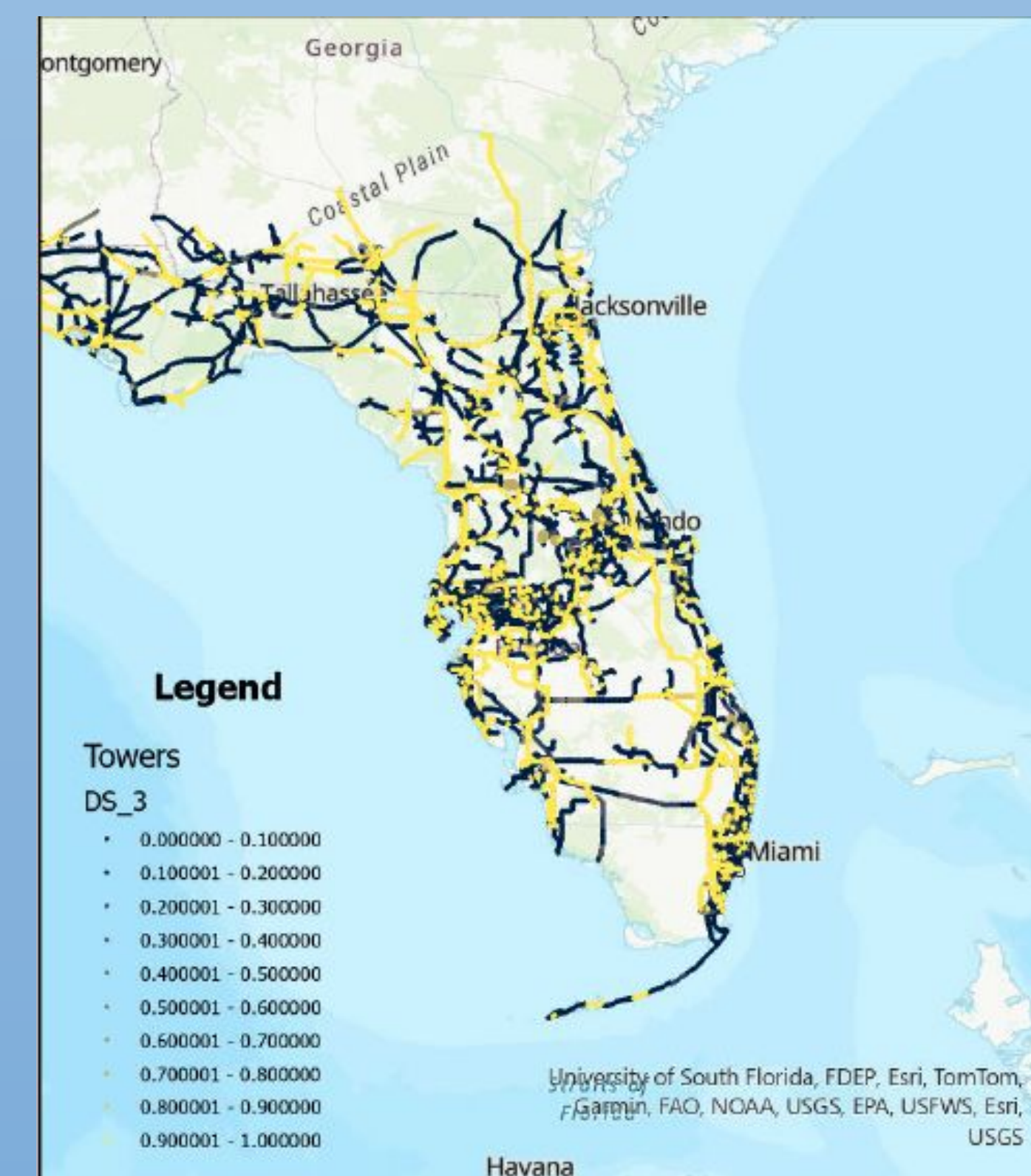
Figure 6: 30-Degree Wind Direction Damage States
