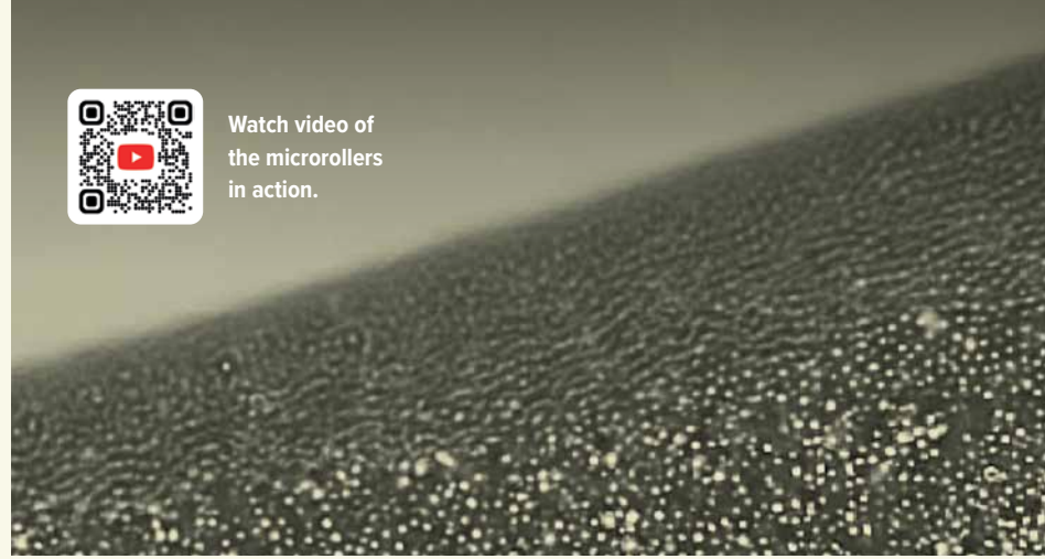
A time-lapse image of microrollers flowing uphill from left to right. A magnet rotates nearby applying torque to each individual particle resulting in a flow that behaves just as granular media does, but flowing uphill.
