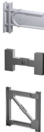
The atrium of Shanghai’s Jin Mao Tower (photos of interior details at right) is the world’s highest at 650 feet. Below (top to bottom): Sarkisian’s Pin-Fuse Frame, Pin-Fuse Joint and Link-Fuse Joint.
