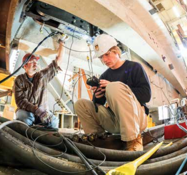
Yen Fellowship recipient Tsampras (above, with ATLSS lab manager Darrick Fritchman, left) is developing an earthquake-resistant building system. Insulation in a plastic hinge (right) shows the effects of spalling from simulated earthquake loading.
