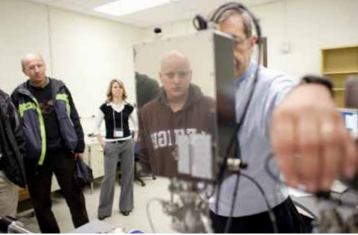
Research scientist Alfred Miller (above) demonstrates the HS-LEIS (left, detail). The instrument fires noble gas ions at the surface of a sample (diagram below) and determines the identity of the surface atoms by measuring the amount of energy lost by the ions in the interaction.
