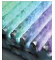
A graded "nanograte" traps a "rainbow" of lightwaves at varying depths, heralding the development of all-optical devices.
