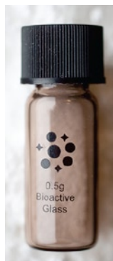
Bioactive glass used as a bone graft substitute.
