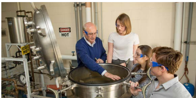
Chemical Engineering majors Francesca Ciccari, Emilia Galka, and James Wilkinson discuss mixing of fluids in an agitated vessel and its effects on heat and mass transfer in the Undergraduate Unit Ops Laboratory.
