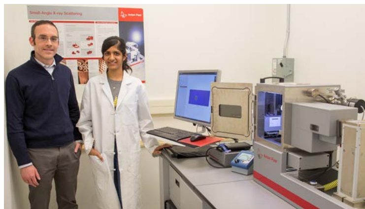
Snyder and student Megha Sharma with small-angle X-ray diffractometer used for non-destructive characterization of particle suspensions to porous materials.
