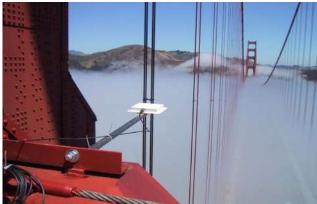
Wireless Sensing for Bridge Monitoring - Courtesy of Dr. Shamim Pakzad
