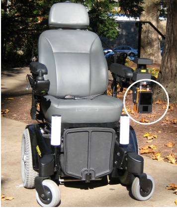
Fig. 1. Prototype smart wheelchair system integrating the the flash LIDAR (encircled white).
