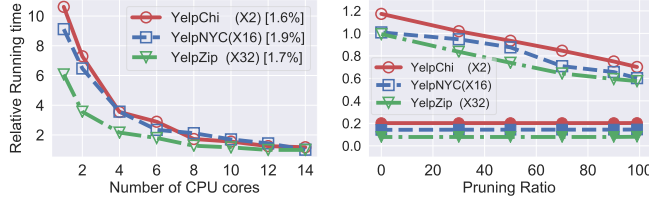
Figure 4. Left the computing time reduces superlinearly as the number of cores increases from 1 to 14. The parentheses enclose the number of hour(s) per unit. The square brackets enclose the running time of GE-L . For example, GE-G takes about 192 hours using one core on YelpZip, while GE-L costs 3 hours. Right Effect of pruning: as we increase the pruning rate to 99%, the subgraph explanation faithfulness is not degraded (shown by the 3 horizontal lines with solid markers), while the running time is reduced by 1/3.
