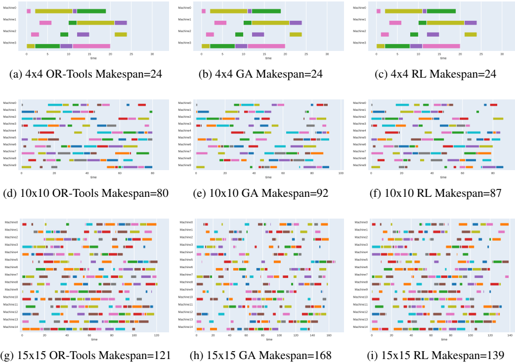
Figure 5: Example solutions for the classic JSP ( \lambda = 0 ) problem, Gantt diagrams. On the left, the optimal solutions computed with OR-Tools; on the center, the result of the Genetic Algorithm and on the right, the results obtained by the RL model with a sampling technique.
