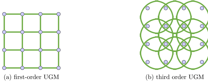
Figure 2: Illustration of clique configurations in a first-order UGM and a third order UGM for image restoration.
