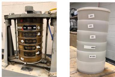
Figure 1. Left Panel: CAWST (hand-held) field sieves, Right Panel: laboratory sieves
