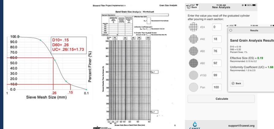
Figure 3. Left Panel: example computer-drawn PSD and ES and UC determination, Center Panel: Hand-drawn PSD Graph paper (included in CAWST BSF Manual), Right Panel: screenshots from CAWST Biosand Filter Sand (BSF) App (currently not available in US Apple App Store)
