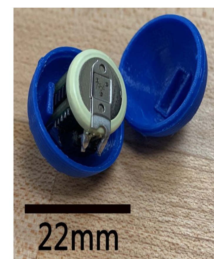
Figure 3: Data logger encapsulated in 3D printed cartridge to keep a water tight seal.
