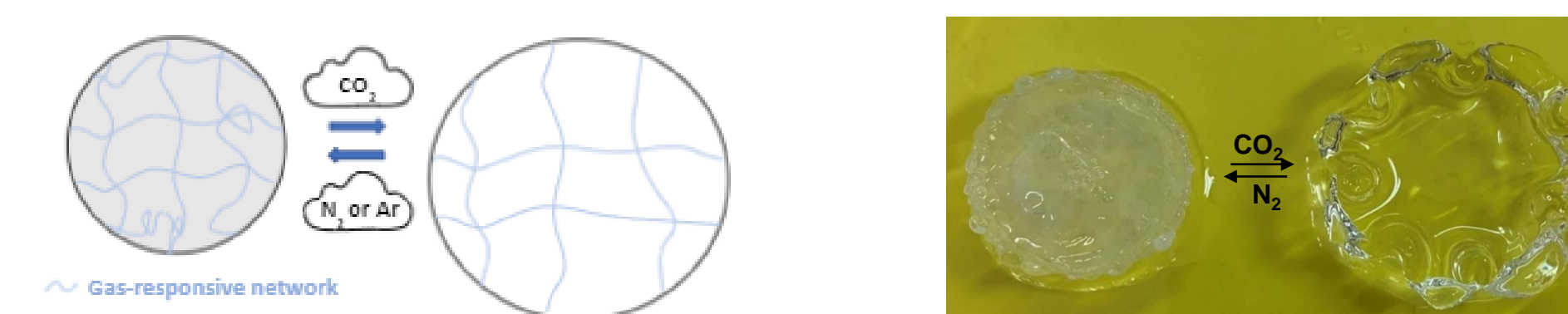
Figure 6: Gas-responsive network swelling and collapse.
