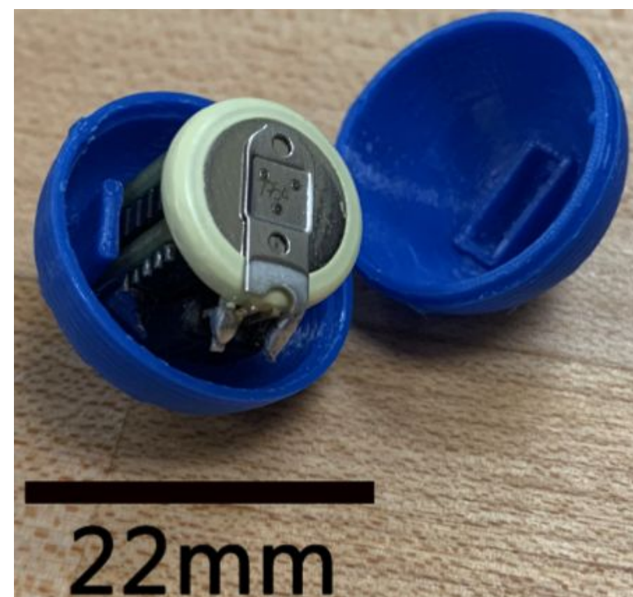
Figure 3: Data logger encapsulated in 3D printed cartridge to keep a water tight seal.
