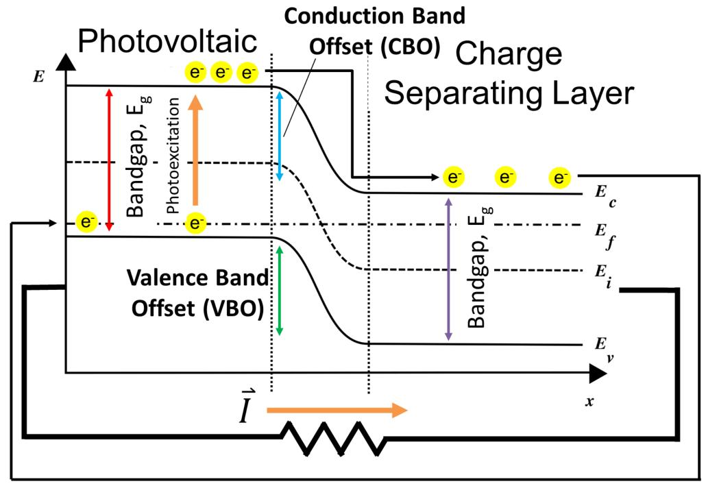
The diagram to the left shows the alignment of the valence bands (EV, valence electrons' "ground state") and conduction bands (EC, first excited state) in such a device. Important parameters for the operation of the device are labeled.
