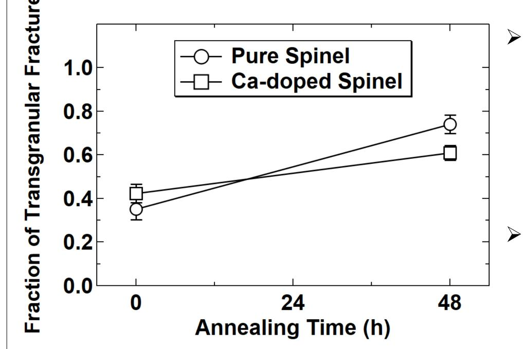
There is a quantifiable difference in transgranular fracture with the addition of Ca as a dopant. Preliminary results show a statistically significant difference in Y-doped samples.
