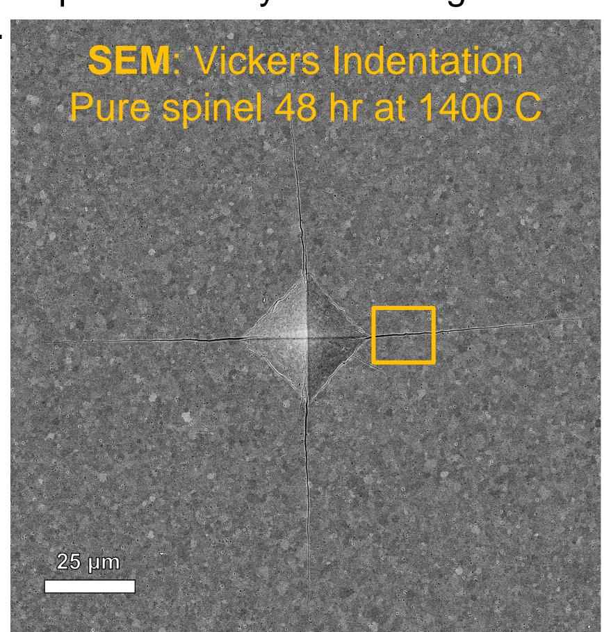
grains (intergranular). The ratio between these two fracture paths was counted along the crack using horizontal slices through the crack. The more transgranular fracture occurs, the stronger the grain-boundaries are assumed to be.
