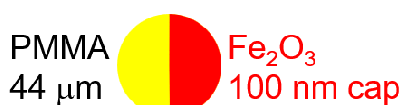
Fig. 2 Janus particles that roll when forced by a rotating magnet 2 .
