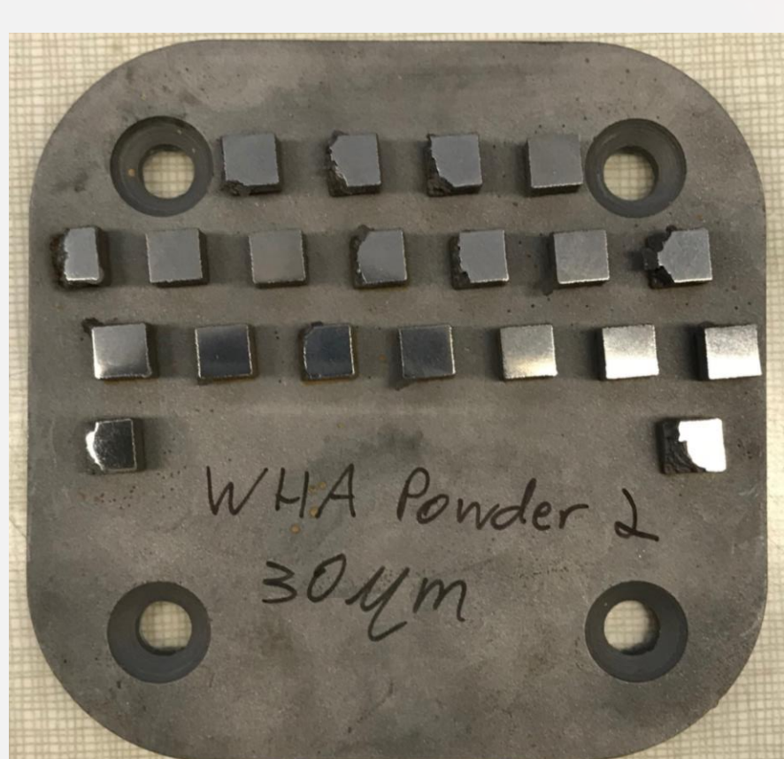
Figure 3. WHA Powder 2 cubes, printed on steel build tray with 30 µm layer thickness.
