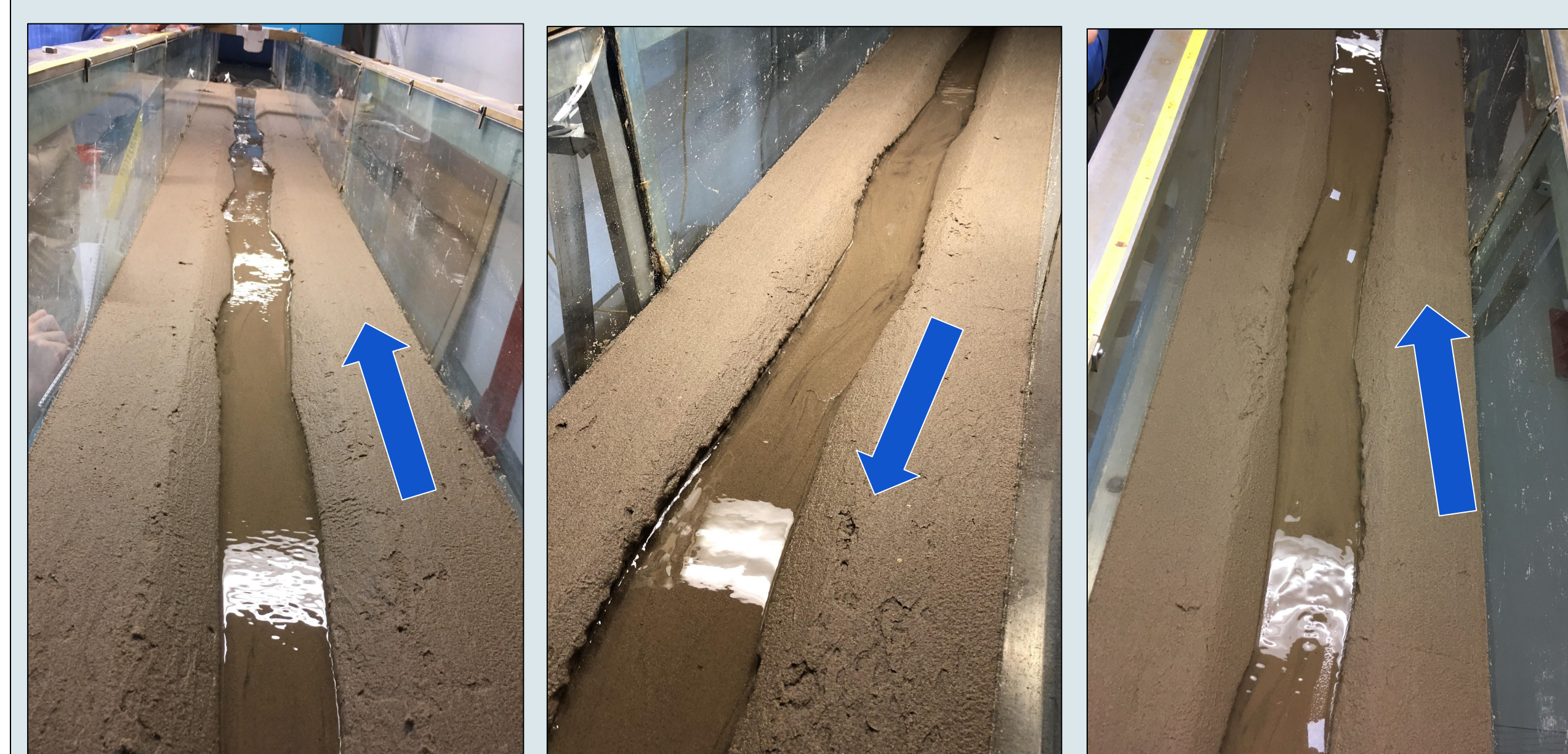
Meandering patterns present in the channel, caused by a reduction in downstream slope. Due to a lack in constant sediment feed upstream, the geometry of the channel is formed purely from the scouring of the sloped banks. The blue arrows denote flow direction.
