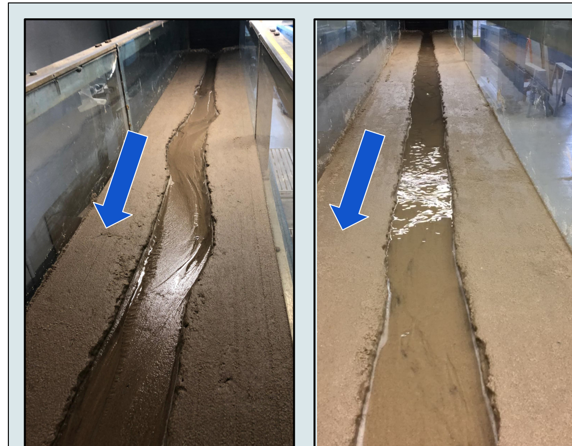
Meandering patterns produced by the addition of a metal obstruction downstream (left). Channel is straight without metal obstruction (right). Blue arrows indicate flow direction.
