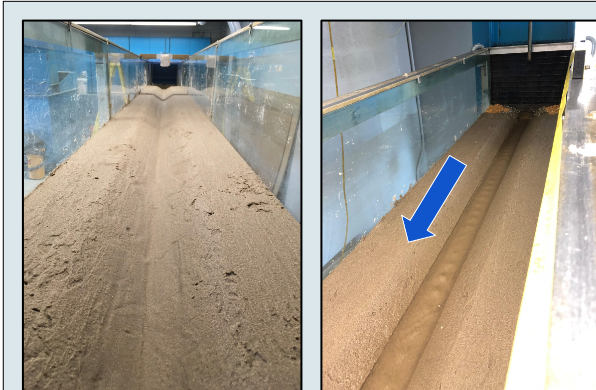
Image on left is initial trapezoidal channel formation, with no flow. Image on right is when flow has begun and erosion is not significant. Blue arrow indicates flow direction.
