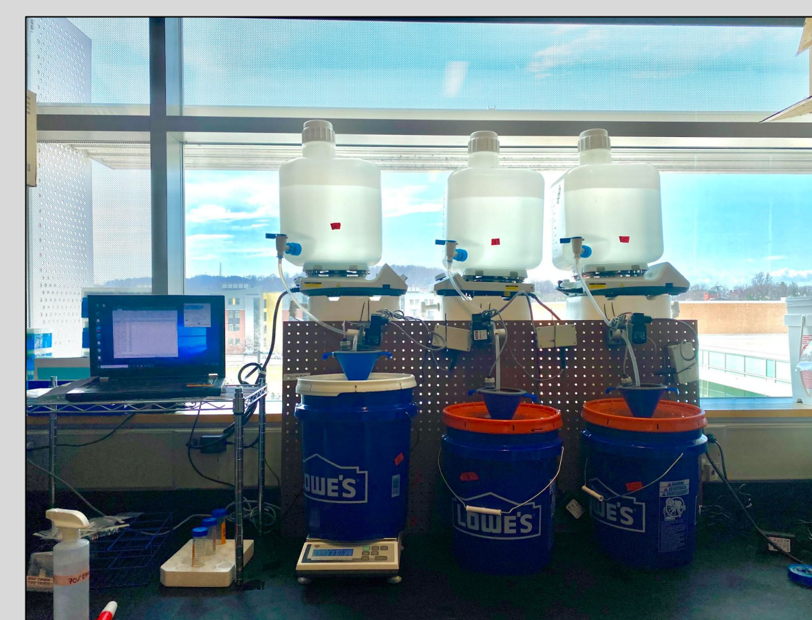
FIG 5: Filtration apparatus during testing of the silver-coated filters
