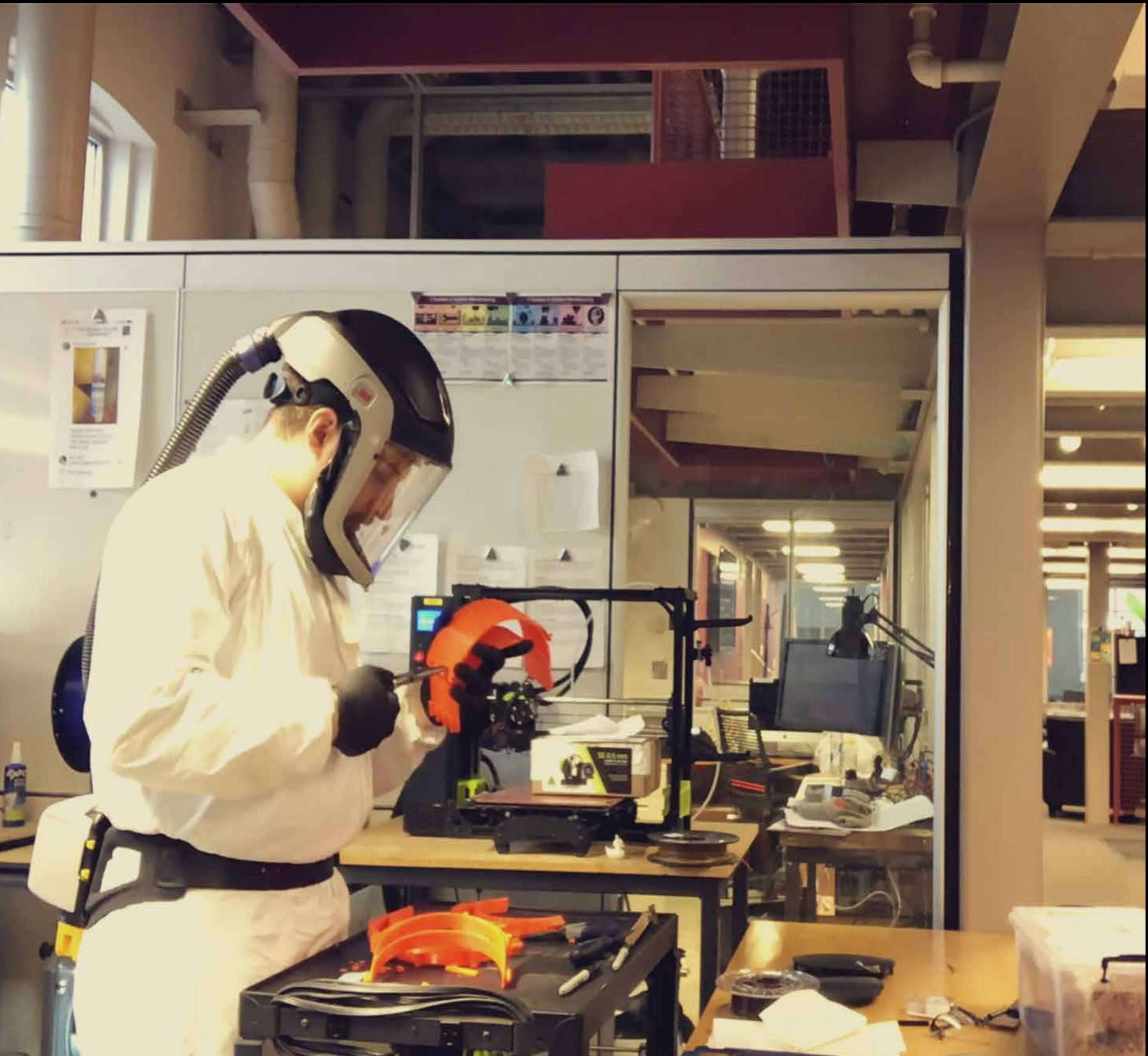
Additive manufacturing coordinator Trevor Verdonik, donning a full suit of protective gear as a precaution against spreading germs, works on face shield components in Wilbur Powerhouse.
