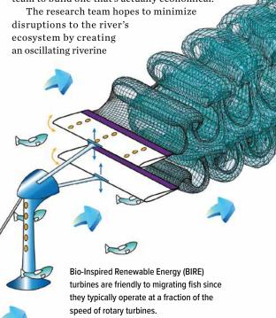
turbine that moves vertically at a slower rate compared with existing rotary river turbines. Sensors in the system will allow it to adapt to natural changes in the river's depth and maintain steady energy production.
